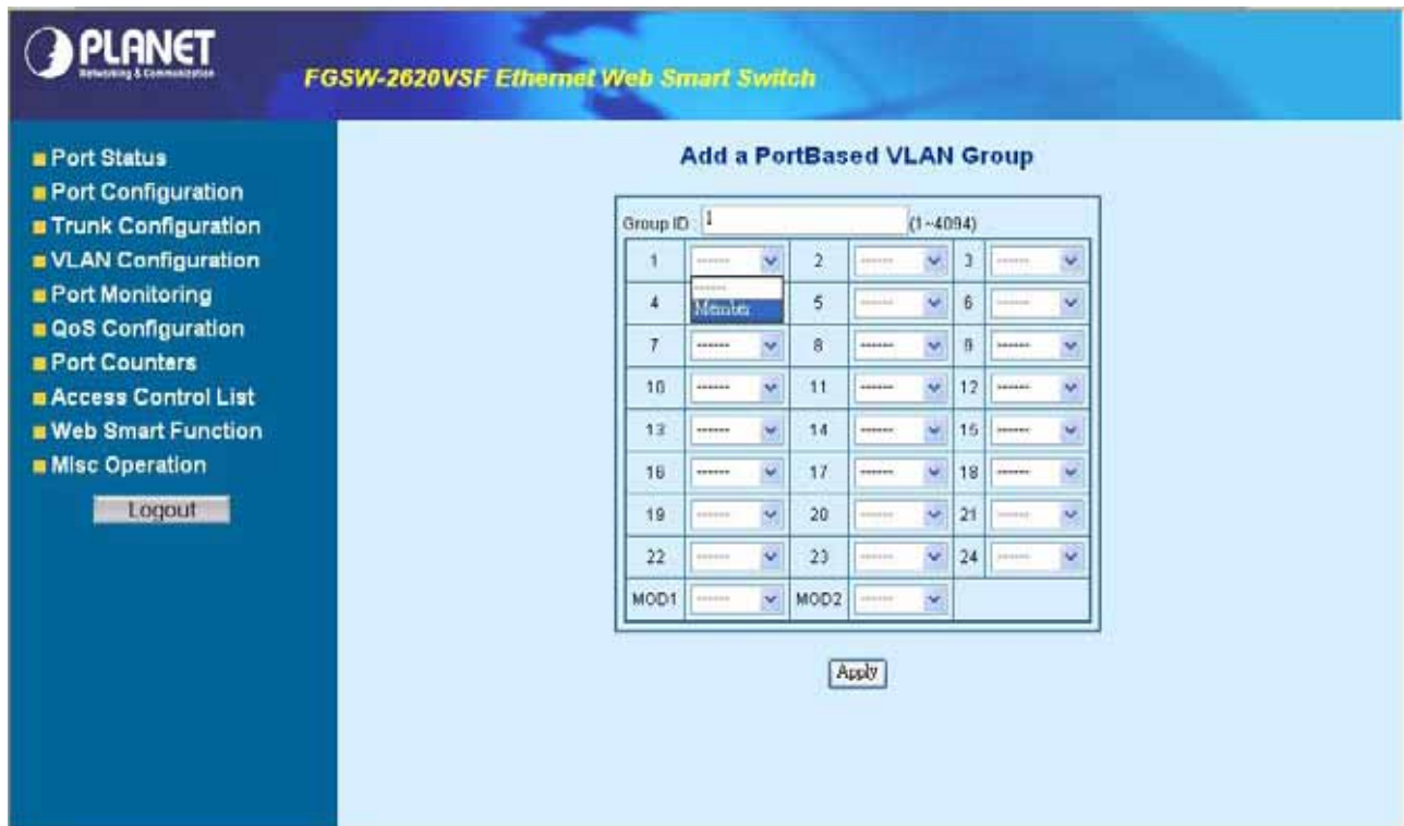
Figure 4-14 Port-based VLAN Setting Web Page screen
